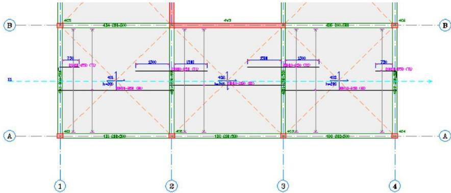
We specified the bar sizes which Orion can use in slab design earlier (see “Defining Materials” on page 15 .) You can also control the slab bar spacing range that will be applied by picking Settings / Slab Design Settings / Steel Bars.
