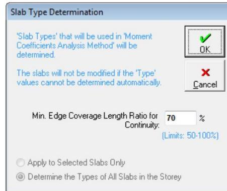
3. Click OK to proceed. Orion determines the slab types.
