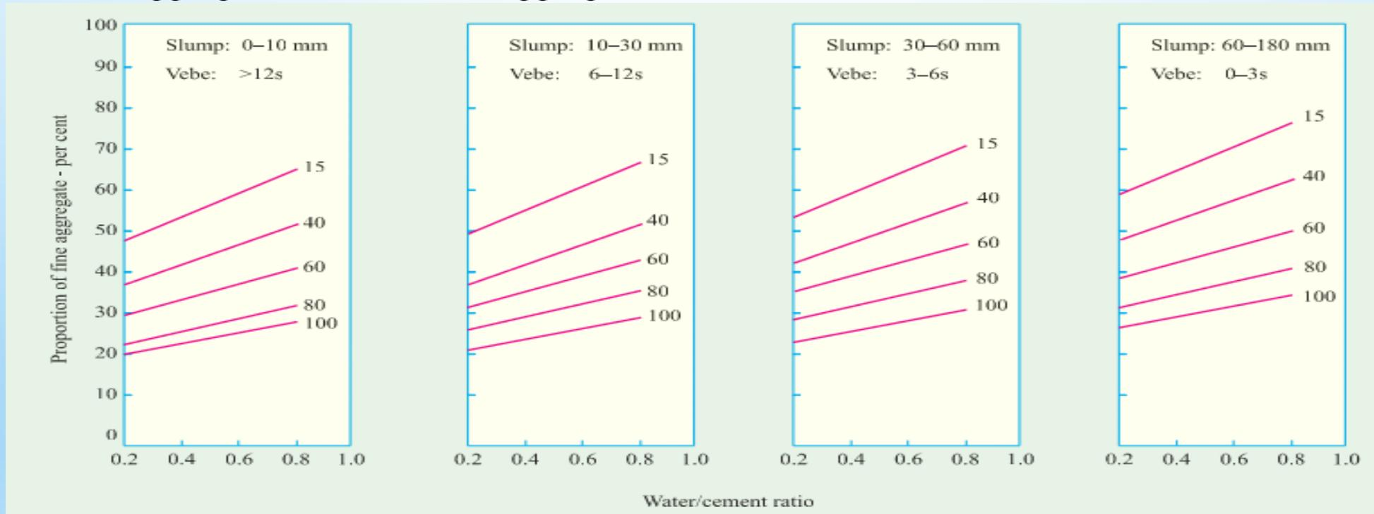
Figure 4: 10 mm coarse aggregate size
