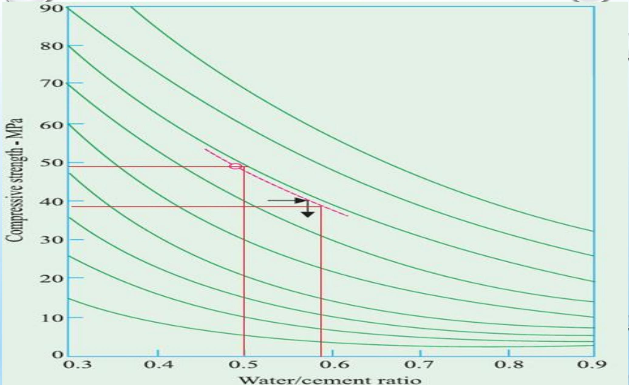
Figure 2: Relationship between compressive strength and free water/cement ratio.
