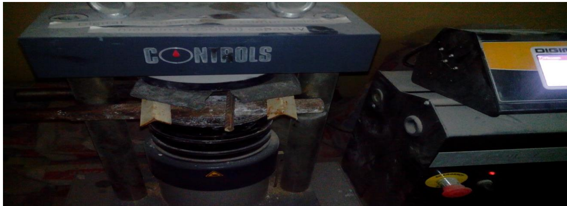
Figure 3: Mortar prism during flexural strength test
