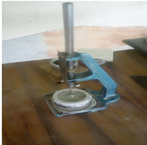
Figure 1: Determination of Setting Time using Vicat apparatus
