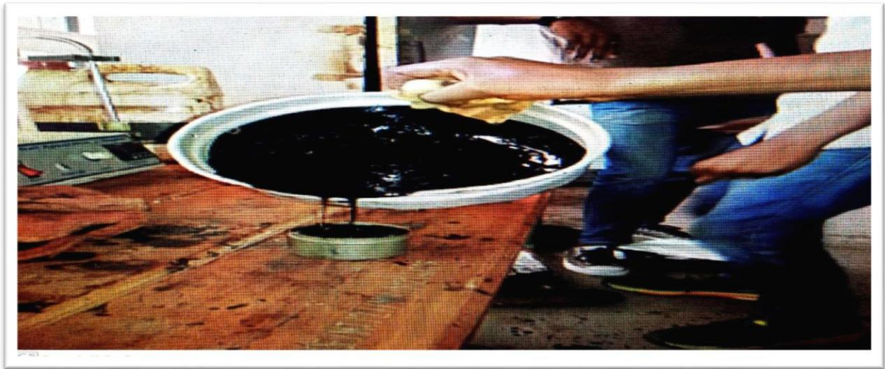
Fig. 1 Shows Bitumen While Preparing the Penetration Samples.
